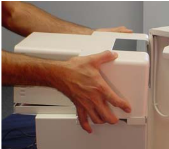
Install printer by allowing front section to rest in place, then lower the rear section into the tray.
