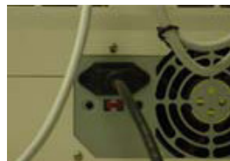
AC Power Connection
