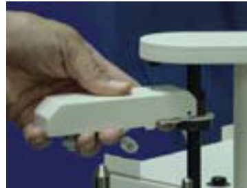
Hold Pick Arm in Place & Connect RJ12 Connector Step 2
