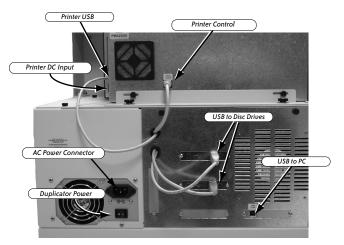
2 Plug one of end of a USB cable into the connector labeled USB to PC on the back of the duplicator cabinet. Plug the other end of the cable into a USB 2.0 port on the selected Macintosh host computer.
