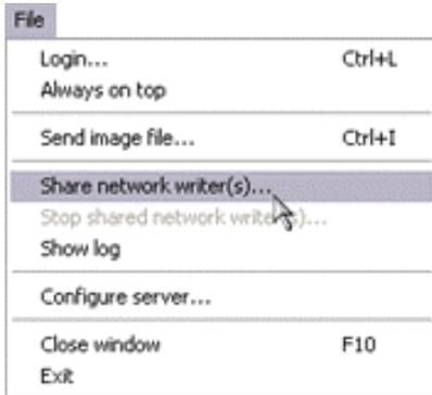
After the Padus Remote Console has started, you need to start the Network Server service. This can be done by going to *File -> Share network writer(s)...* (shown above). This will open the primary configuration window for the Network Server service.
