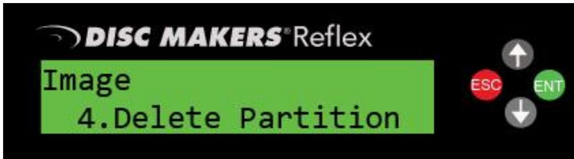
Scroll through the partitions that you currently have on the machine using the
