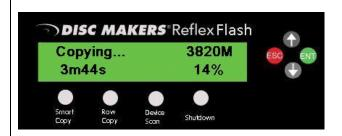
The system will scan the Source flash device and proceed with the Copy process immediately. (Shown on the left)
