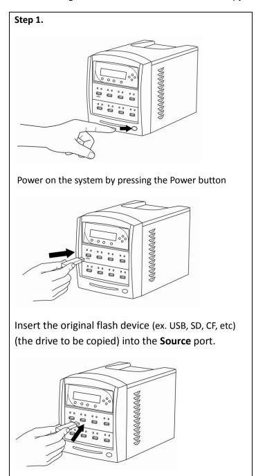
Insert empty target flash devices (ex. USB, SD, CF, etc) into the other **non-Source** ports.
