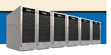
The Reflex DC unit will allow you to connect multiple units in a daisy chained configuration. The first unit in the chain controls all drives within the connected towers. This will save time by allowing more discs to be copied in a single pass.
