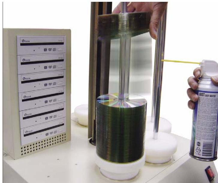
Figure 1-1 Using Canned Air to Reduce Static
