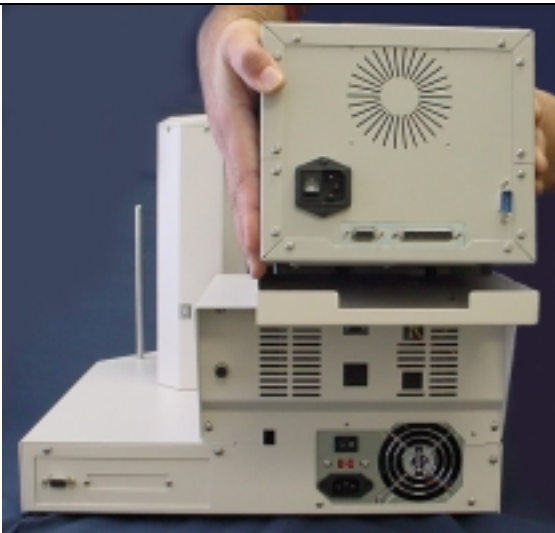
Step 5 Place the PowerPro into the Tray with the Front of the Printer being inserted first, then allow the back end to drop into the tray.
