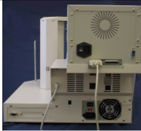
Step 6 Connect the AC Power cord, the Printer Control Cable and the Parallel cables as required.
