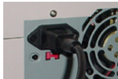
AC Power Connection
