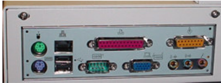
Rear View of Connections
