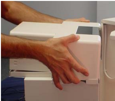
Install Printer by allowing front section to rest in place, then lower the rear section into the tray.
