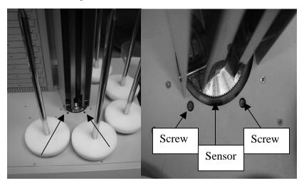
2. Loosen the two sensor retainer screws. (You may need to slowly and carefully move the arm column to obtain clear access to screws and sensor)
