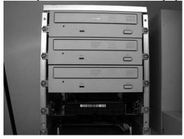
9. Once the screws are removed the drive will slide towards the front of the unit. Once the drive clears the housing gently removed the ribbon cable by grasping the black connector plugged directly into the drive at the end of the cable.
