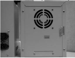
5. Once the screws are removed carefully slide the housing slightly towards the rear of the unit.
