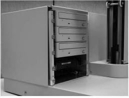
6. Once the housing is slid back approximately an inch lift the housing directly up. It should slide off easily.
